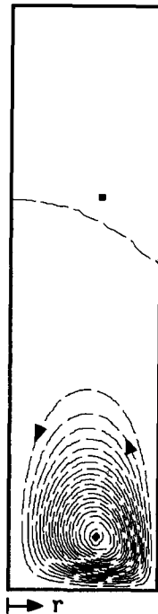
Fig. 4. Level lines of the dimensionless stream function \Psi in the meridional plane for an aspect ratio of four. \blacksquare = 0.0001543 \times 10^{-4} , \blacklozenge = -4.129 \times 10^{-4} .
